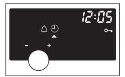
To **select a function**, turn the multi-function selector until **triangle** ▲ **is underneath the required symbol** in the display of the function you wish to make changes to.
